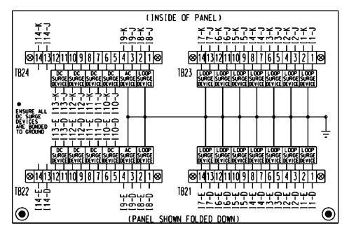
For base mounted cabinets, mount surge protection panels on the left side of the cabinet as viewed from the rear. Attach each panel to the cabinet rack assembly using bolts and make it easily removable. Mount the surge protection devices in vertical rows on each panel and connect the devices to one side of 12 position, double row terminal blocks with #8 screws. For each surge
